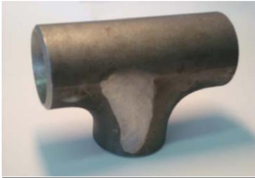
**Figure 1:** Steel work-piece with partially grinded surface.
