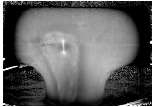
**Figure 2:** Phase image of the work-piece shown in Figure 1, the crack is very well visible at the grinded part.
