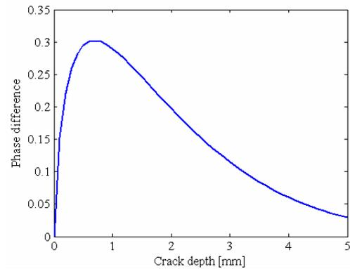
**Figure 4:** Additional phase around a surface crack depending on its depth.
