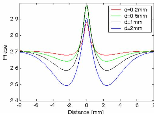
**Figure 3:** Calculated phases around surface cracks with different depth values at the position of '0'.
