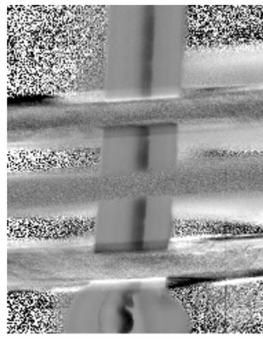
**Figure 6:** Phase image of a non-magnetic wire. The surface crack (cold lap) becomes very well visible through a lower phase value.
