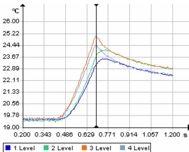
**Figure 5:** Timing graphs for inductive pulse heating at some points of a non-magnetic material. Level '1' and '2' are located in the region of a surface crack, '3' and '4' are at the surface without failure.
